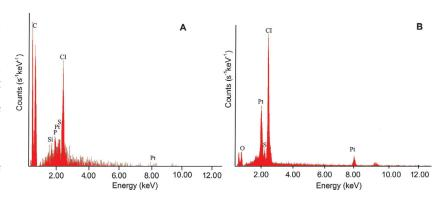
Fig. 4. Energy-dispersive X-ray (EDX) analysis of dark (A) and light (B) areas of the specimen illustrated in Fig. 3, confirming the adsorption of platinum chloride ions to the light areas on the sorbent.
