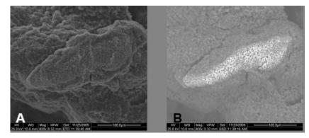
Fig. 3. Scanning electron micrographs of the sorbent surface after incubation with platinum ions to illustrate both the biological (A) and non-biological (B) components of the specimen.
