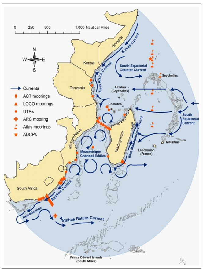
ACT, Agulhas Current Time-series. UTR, underwater temperature recorder. ARC, Agulhas Return Current refreence station. ADCP, acoustic Doppler current profiler.
