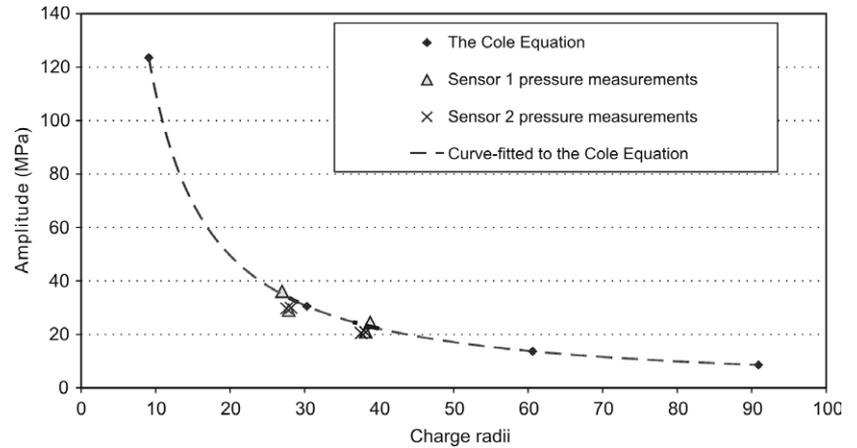
Fig. 8. The amplitude of the pressure (MPa) measured in this study, versus the standoff distance (charge radii), compared to that obtained by the equation given by Cole.<sup>2</sup>
