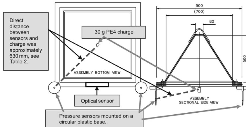
Fig. 1. Mechanical detail for Events 1–3 of this experiment.
