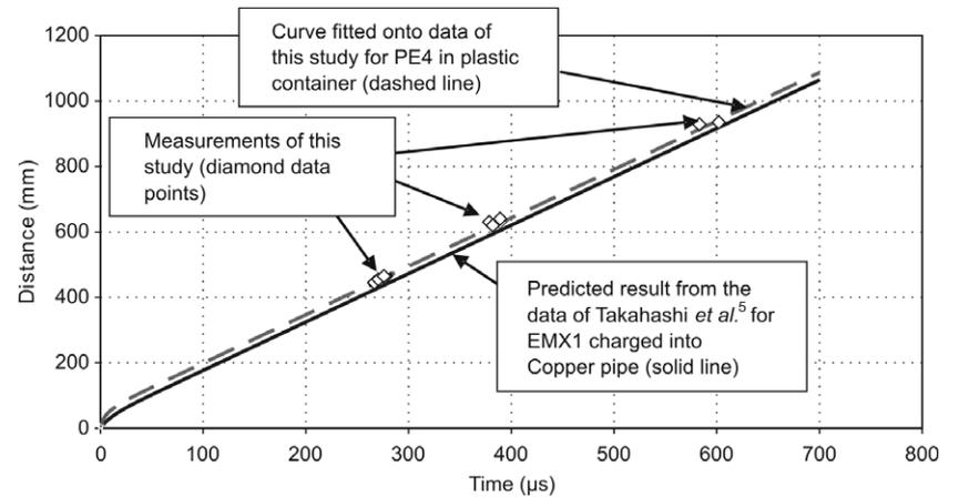
Fig. 13. A plot of the distance travelled by the shock wave versus the time taken for that distance to be travelled, obtained by measurement in this study and by the equation of Takahashi *et al.*<sup>5</sup>
